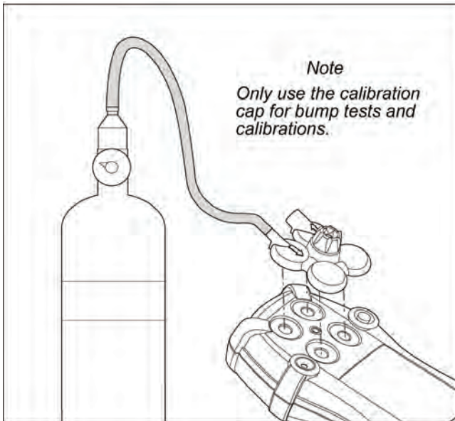
Figure 11. Connecting the Gas Cylinder to the Detector
